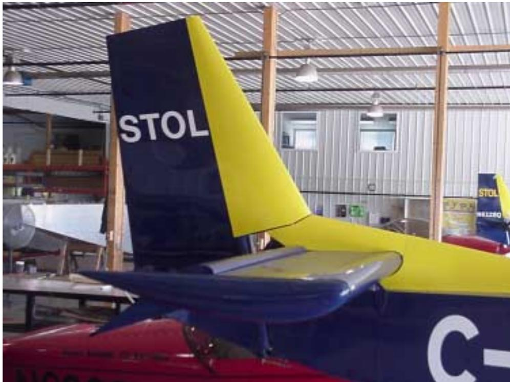
Note the fin on the fuselage and stabilizer is but to match the leading edge of the rudder.
