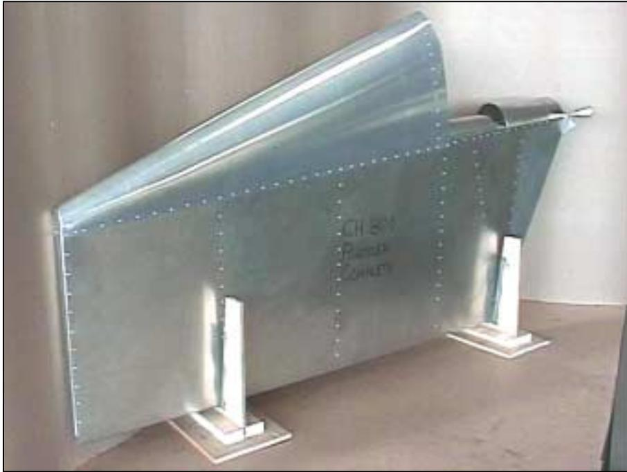
The completed rudder assembly
