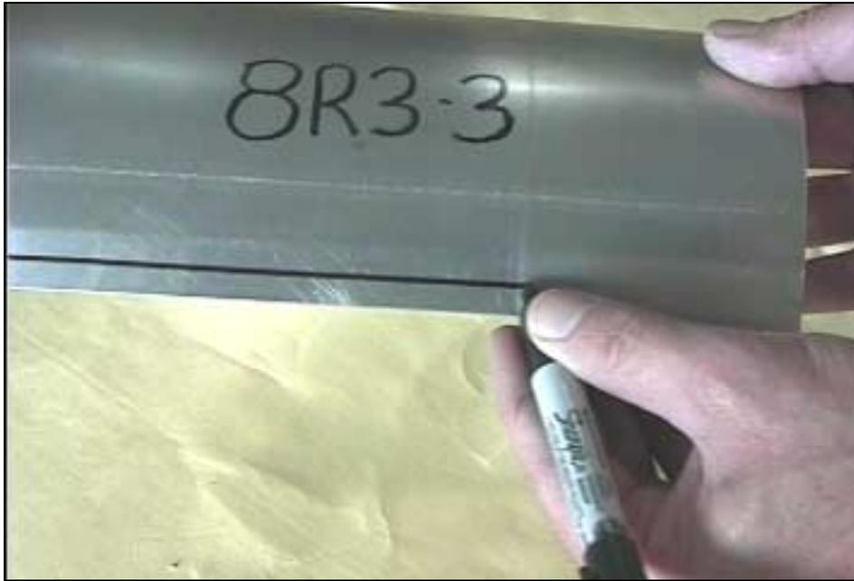
Mark a rivet centerline down one side of each of the fairings, 10mm from the edge.
