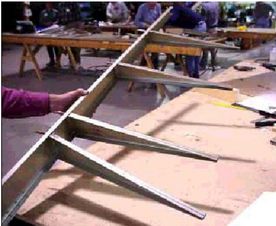
Rear ribs on spar.
