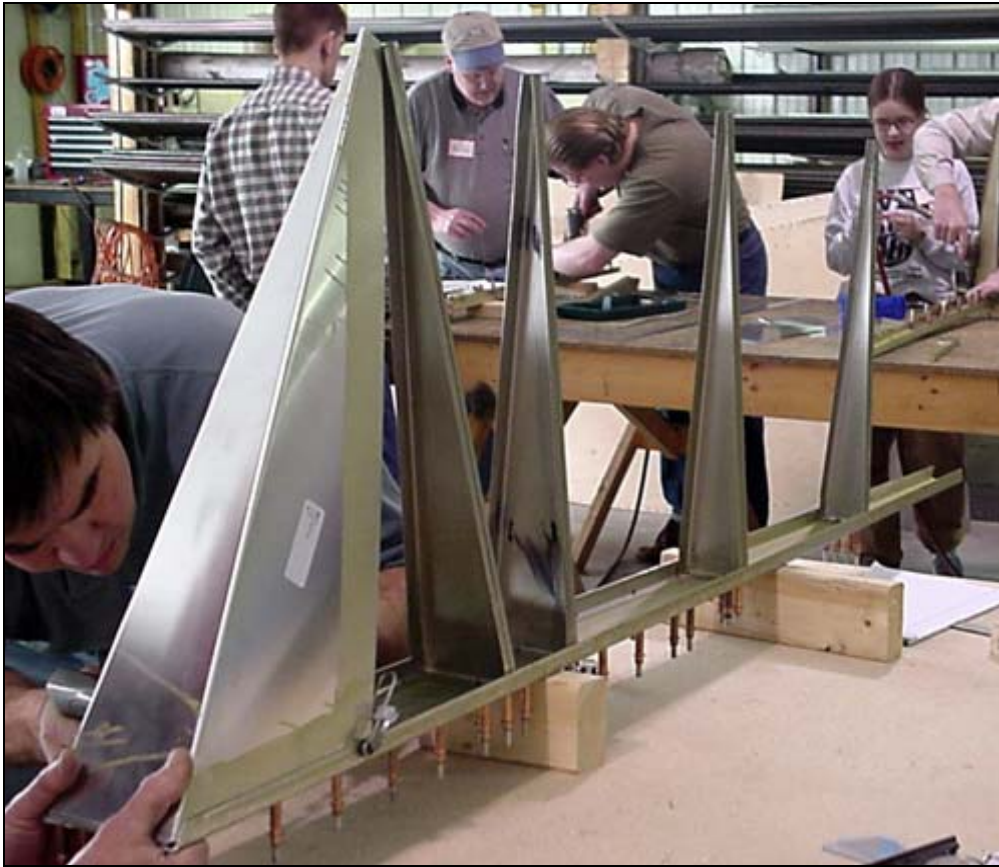
Rear ribs on spar.
