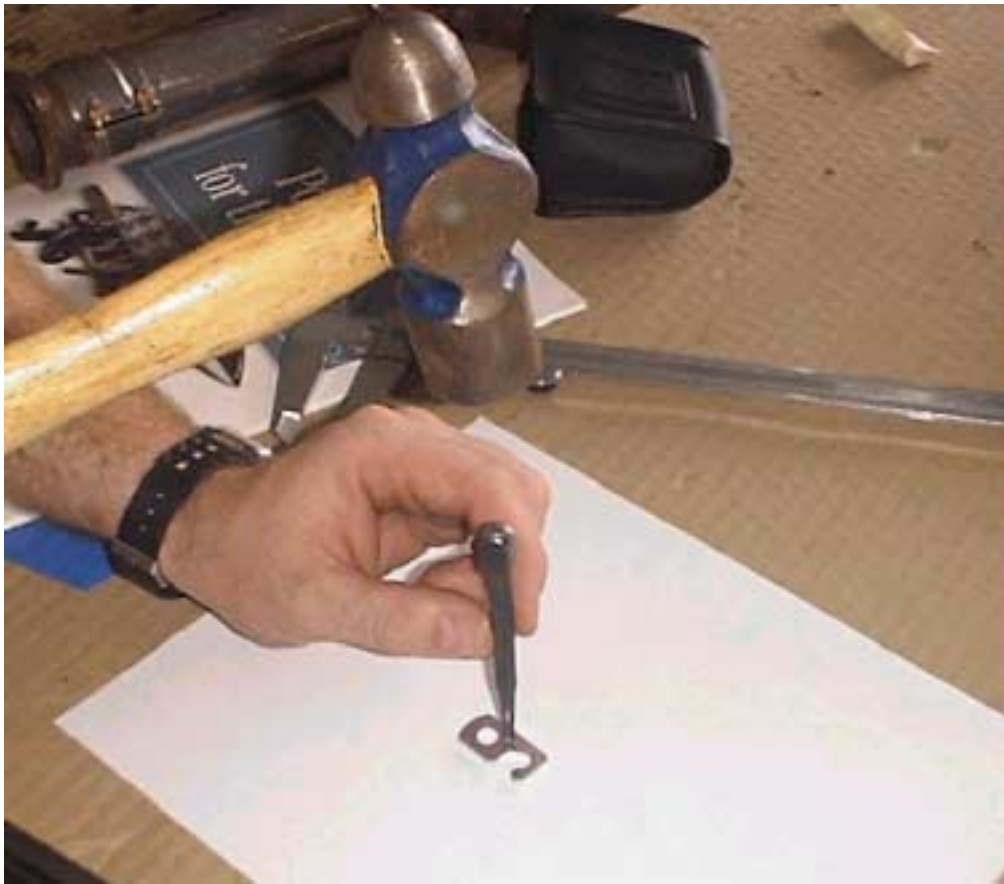
Center punch the hole in then drill with a 1/16" drill bit.
