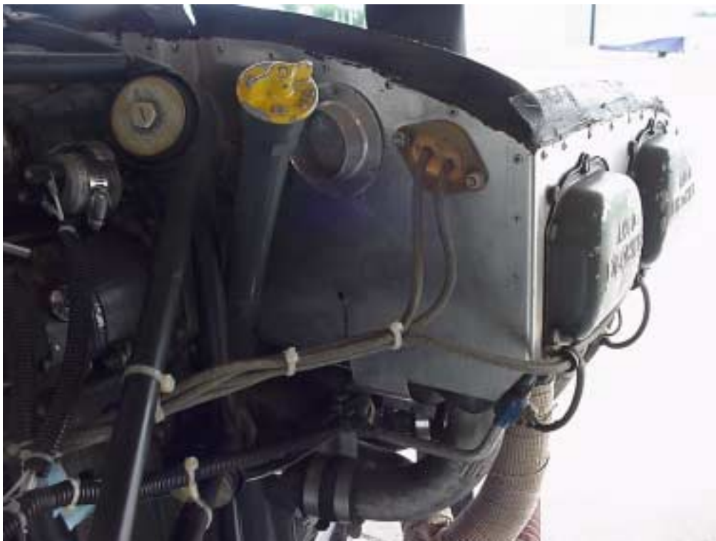
Note the routing of the magnito wires on the right side of engine.
