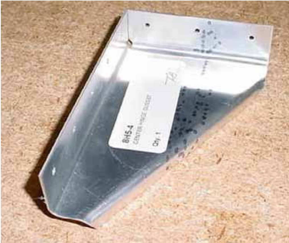
8H5-4 gusset with predrilled holes.
