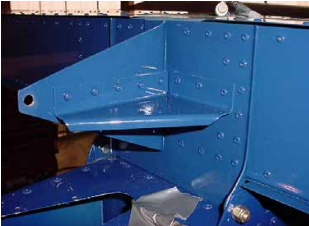
8H5-4 gusset with predrilled holes.
