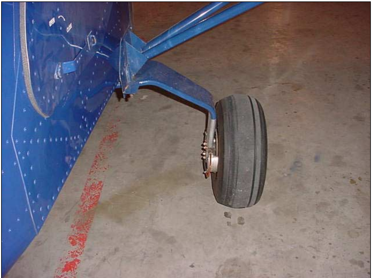
Front view of left wheel (Murphy wheel with dual calipers used up to Jan 2003, Ref drawing 8LS-1 for gear cutout for murphy wheels only)
