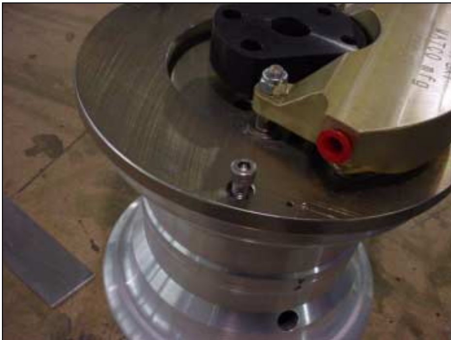
Unscrew the 3 cap screws to remove the disk brake
