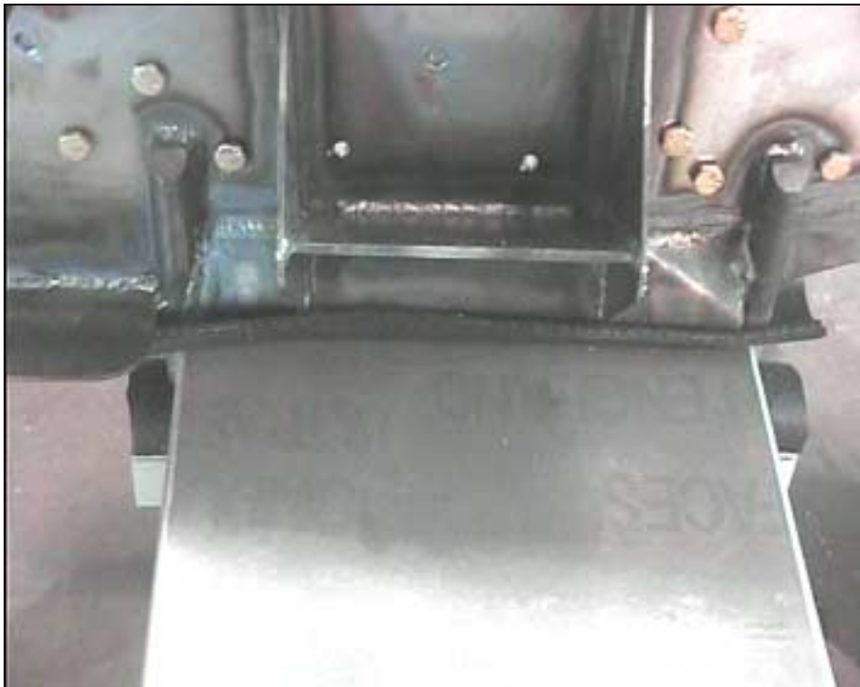
Bolting the gear to the fuselage.
