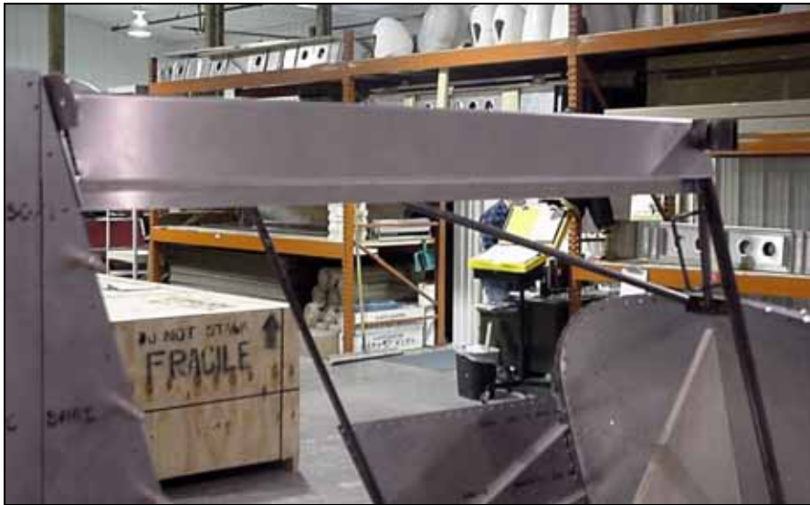
The positioned door sill, right side (8F19-5)
