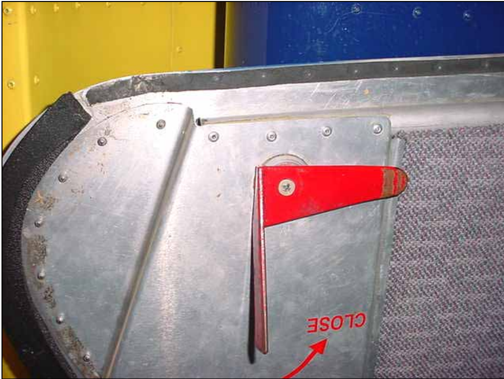
Right door – Bent Lower Tube 8F19-8 Standing under the wing looking up at the bottom of the door.
