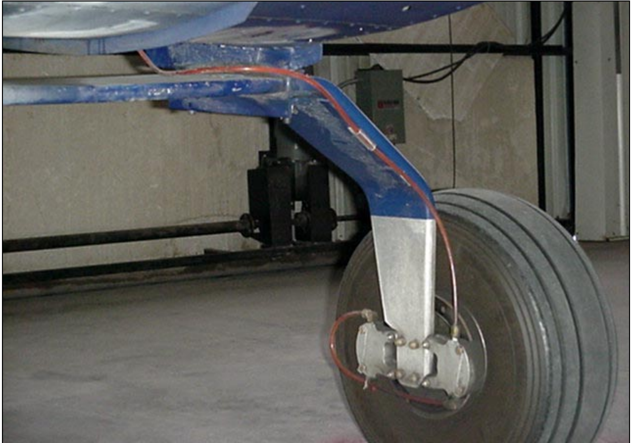
Photo of right wheel, brake line run on the back side of the gear spring.
