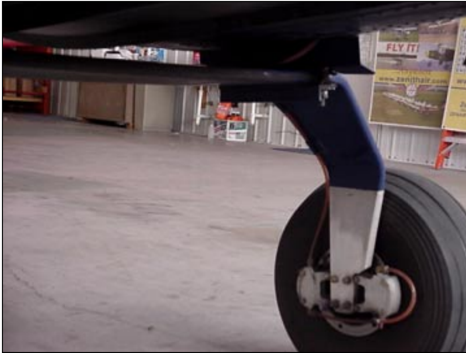
Left wheel with dual hydraulic calipers (photo looking back at the wheel)
