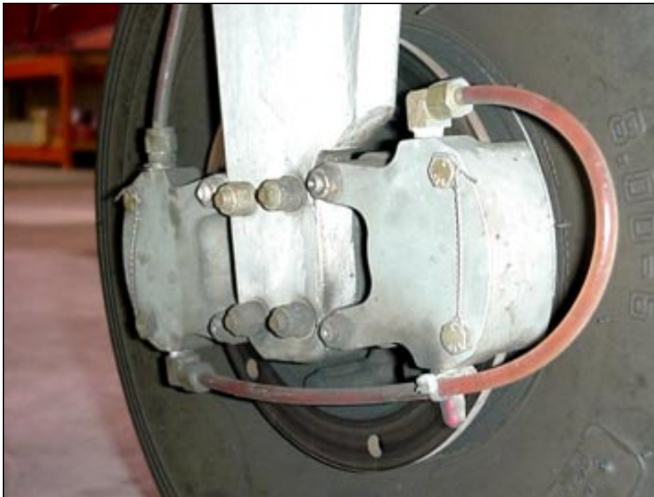
Left wheel with dual hydraulic calipers (photo looking back at the wheel)
