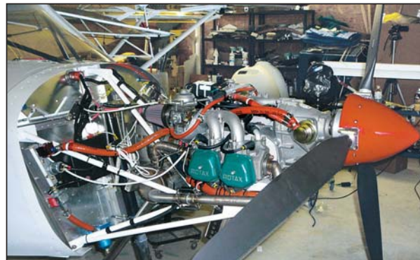
The new Rotax 912 ULS 100 hp with 2,000 hour TBO motor.
