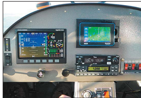
The panel features Dynon D180, Bendix/King AV80R GPS, ICOM A210 and a Garmin GTX 327 Mode C transponder.
