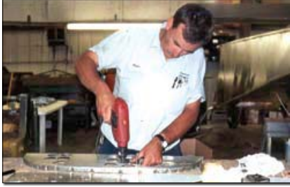
Hand-drilling the panel using a borrowed instrument panel punch took one evening.
