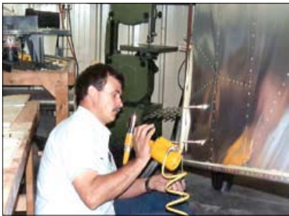
Well along in the assembly (about eight months), the fuselage sections are finish riveted together. The instrument panel form block, a major part of homebuilding, is visible behind Clagg on the table.
