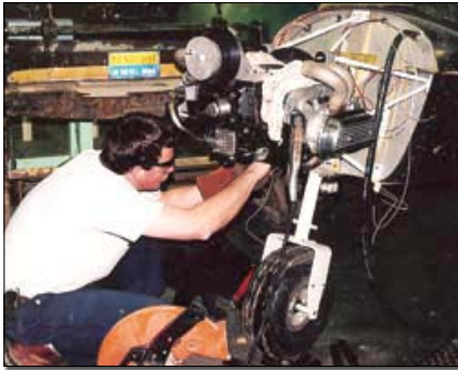
Getting a plan together for the exhaust system. You can see the homebuilt engine mount and the Valley Engineering redrive here.
