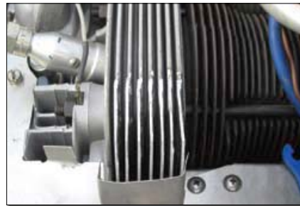
The right cylinder head with the trial or developmental first generation fin extensions. Testing proved the fins were too large, and they were reduced in size and number on the second generation heads Clagg currently flies.
