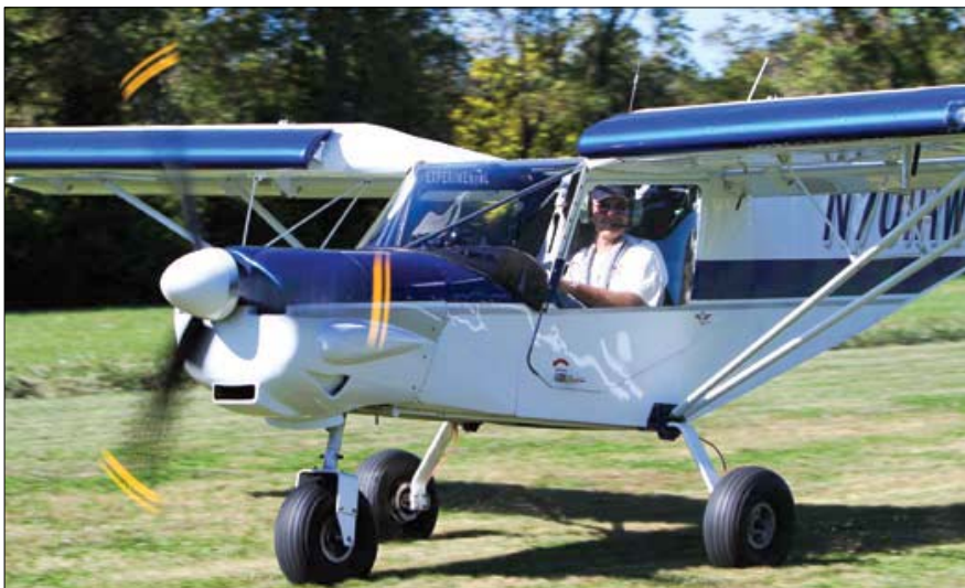
The smile absolutely says it all. After a few engine and prop changes the performance is much better. Climb is 750 fpm, cruise is 90 mph with CHTs around 270°. Reliability has improved enough that Clagg routinely flies to local airports and fly-ins.
