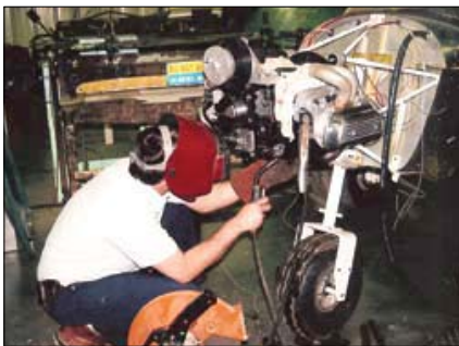
Tack-welding the scratch-built exhaust system. Clagg made almost every part of the plane.
