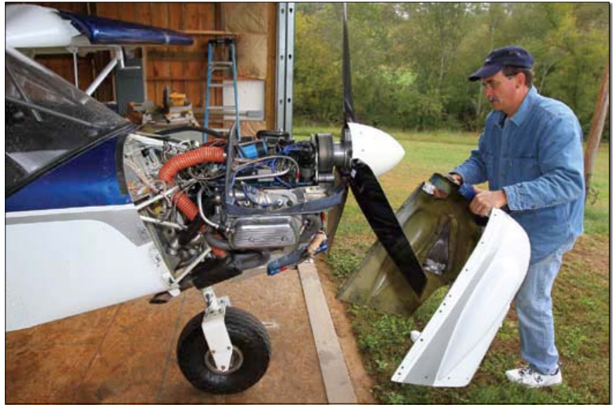
Removing the cowling for a routine maintenance check and oil change takes a few minutes. The engine makes about 102 horsepower at full power, and Clagg cruises at 3900 engine rpm and approximately 85 hp.
