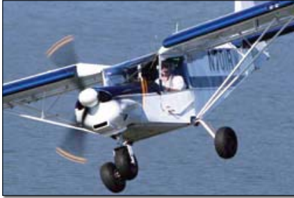
A good view of the scratch-built cowling and 68-inch Powerfin three-blade prop. The oil cooler intake is on the bottom, and the NACA ducts are no longer functional.
