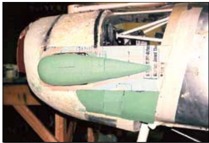
Building up the cowling plug using spray foam, sheet foam insulation and floral foam. The engine is in that mess somewhere. This was the hardest part of the project and nearly brought the build to an end.
