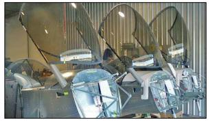
specifically for Sport Pilots. It is the latest model in the Zodiac line of aircraft from aeronautical engineer Chris Heintz, first introduced in 1984. This newest model offers updated features including modern new styling with a larger cabin area and new bubble canopy. Standard features include wing baggage lockers, dual welded aluminum fuel tanks (located in the wings), choice of landing gear configuration (tricycle or tail dragger).
